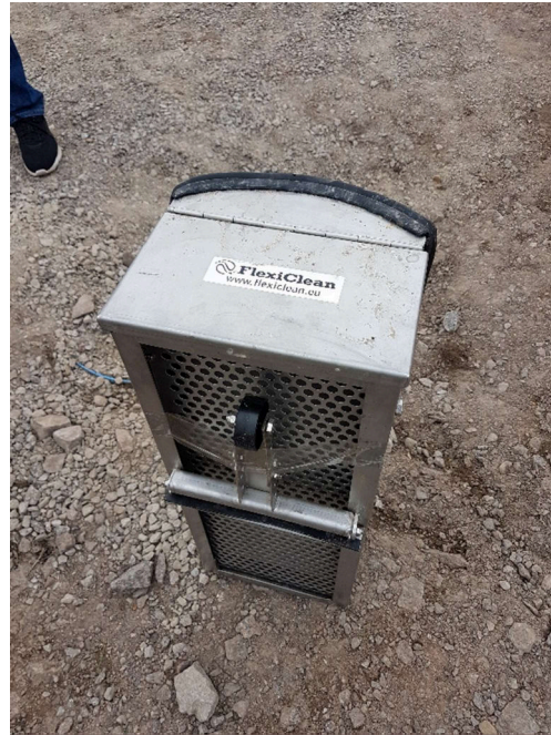
Figure 4. Granulate filter before installation in drain at Bergaviks IP
